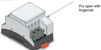
Remove the small plastic shroud on this controller using your finger nail in the top slot of the shroud (see Figure above) and depress and hold the **Discovery Button** for four **(4)** complete flash cycles (i.e. LED cycles **OFF** immediately, then turns **ON** 1<sup>st</sup> time, then a **LONG OFF**, turns **ON** 2<sup>nd</sup> time, then a **LONG OFF**, then turns **ON** 3rd time, then a **LONG OFF**, then when turns **ON** 4th time, quickly release
