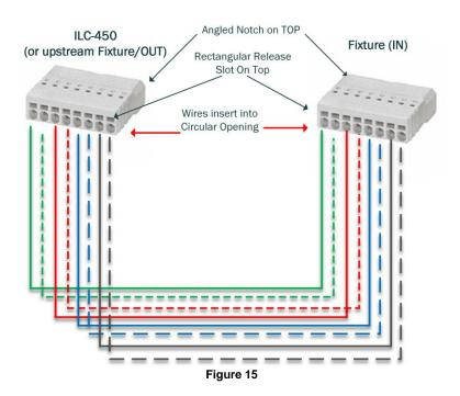
**b.** Make a connection from the "OUT" connector on the 1<sup>st</sup> LED fixture to the second LED fixture and to subsequent LED fixtures according to diagram below:
