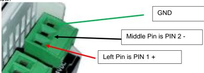
Figure 3 (3-pin power connection)
